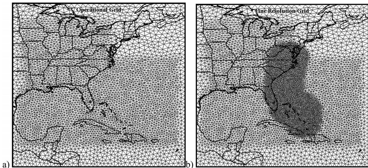
FIG. 5. The OMEGA grid for the low-resolution (LRES) runs (left) and the high-resolution (HRES) simulations (right).
