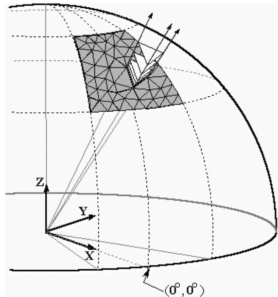
FIG. 2. The OMEGA coordinate system and vertical alignment of OMEGA grid.
