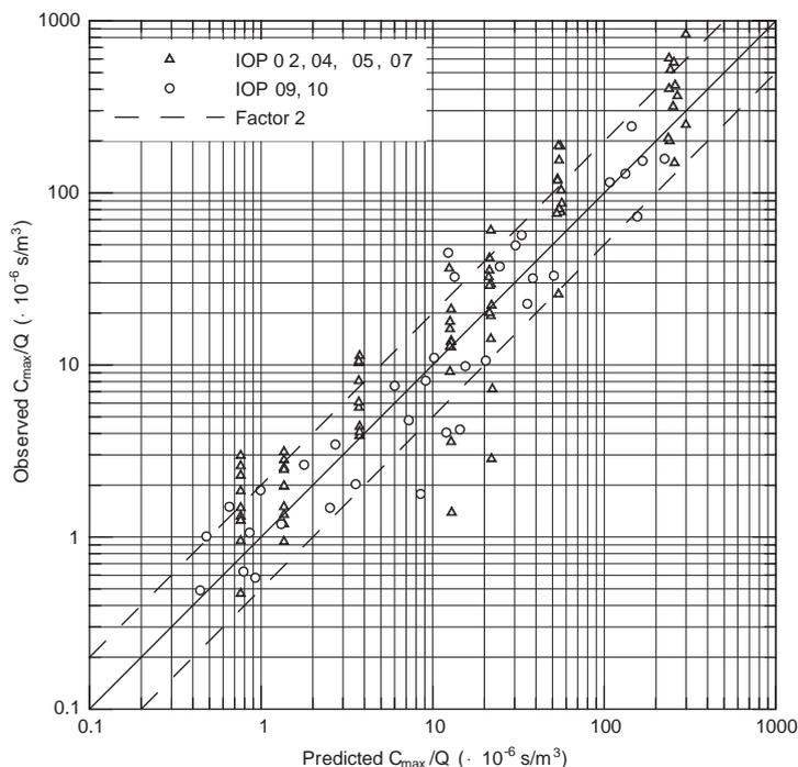
Fig. 5. Salt Lake City Urban 2000 observed and predicted hourly averaged  $C_{\max}/Q$  for all 18 trials for the seven monitoring arcs. The predictions incorporate the  $u$ -dependency in Eq. (12) for  $\sigma_y$ . The triangles represent the “low wind” IOPs 02, 04, 05, and 07. The circles represent the “moderate wind” IOPs 09 and 10. The dashed lines correspond to a factor of plus and minus two agreement.
