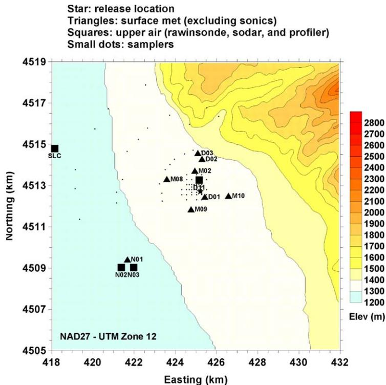
Fig. 1. Map of Salt Lake City domain used in the Urban 2000 study, showing the locations of the release, the surface meteorological monitors, the upper air sites, and the SF<sub>6</sub> samplers. (Map prepared by Joseph Chang.)
