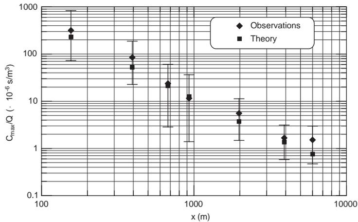
Fig. 4. Salt Lake City Urban 2000 observed and predicted hourly averaged  $C_{\max}/Q$  for all 18 trials for the seven monitoring arcs. The solid symbols represent the averages over all the trials, and the range of the 18 observations is shown as the vertical bar. The predictions represent the simplest “ $u$ -less” model assumptions.
